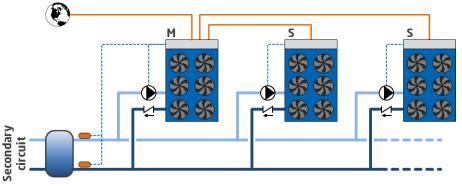
On the basis of the information recorded by the temperature probes installed on the delivery and return manifolds of the system, with the master unit, a capacity request is generated that is distributed among the units connected in the Multilogic network according to settable priority and optimization logics.
