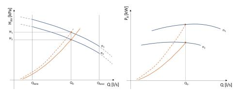
Flowzer VDE is used to automatically adjust the pump speed. As the graph shows, the inverter trips and increases the pump speed if a different condition occurs which would cause an undesired drop in the flow rate (e.g. operation of an external dry cooler). This is a more accurate solution than the VP option alone as it always provides for the water flow (Qd) required by the design conditions.
